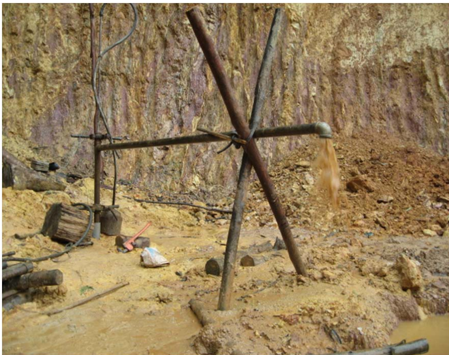
Picture II-3: Water withdrawing slug test at drill hole LK1-T18A
