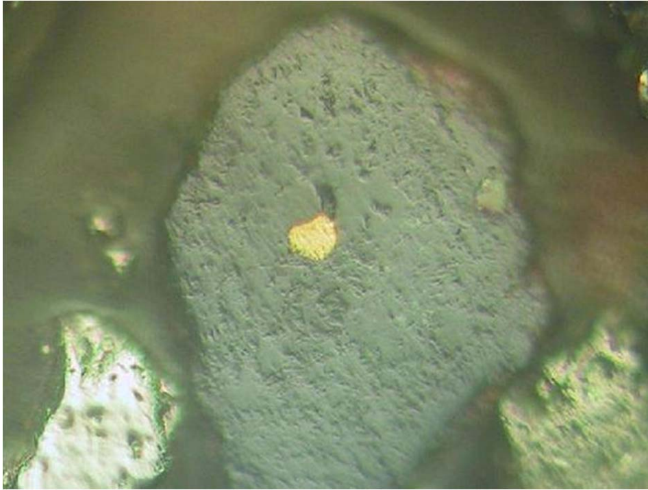
Photo 2. Gold in limonitized pyrite of ore body (TQ) III. Exaggeration: 500 times
