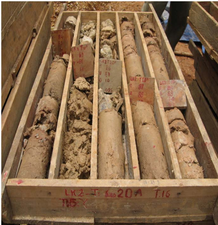
Picture II-2: Drilling core sample LK 2-T20A
