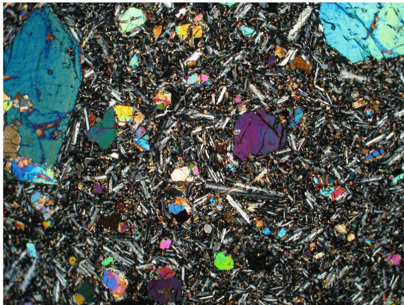
Photo II – 10: Basalt olivine through a thin section (Sample XX. 026, Nicol: N^+ , Zoom: 240 x )
