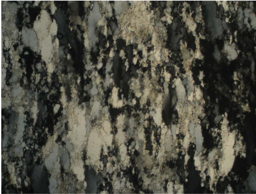
Photo II – 7: Fine - grained quartzite with oriental structure (Sample XX.216/1; Nicol: N + ; Zoom: 480 x )
