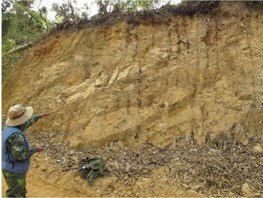
Photo II – 7: The light colored sandstone layer and sandwiched layers of siltstone, sericite shale. VL. SK - 036. Picture Do Quoc Binh
