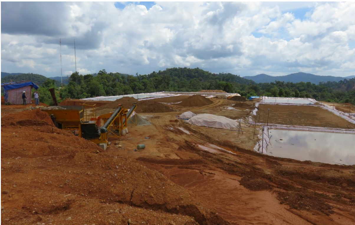
Figure 9: Small scale crushing and leaching of oxide gold ore
